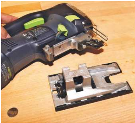
▲ The base comes away quickly and easily for changeovers
